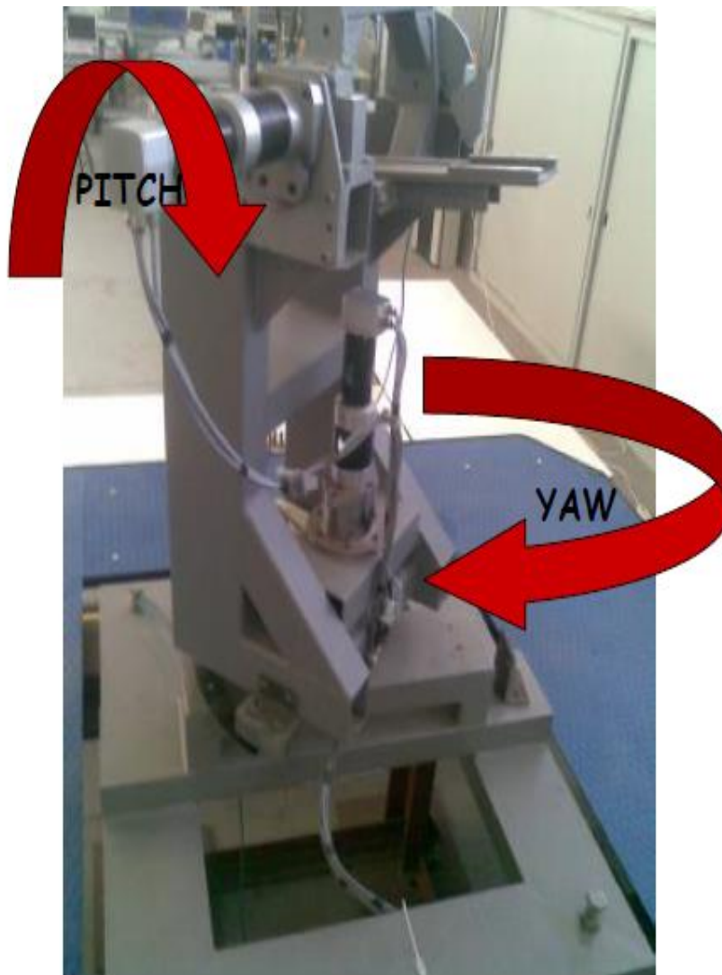
Figure 3: Two axes platform with motors
